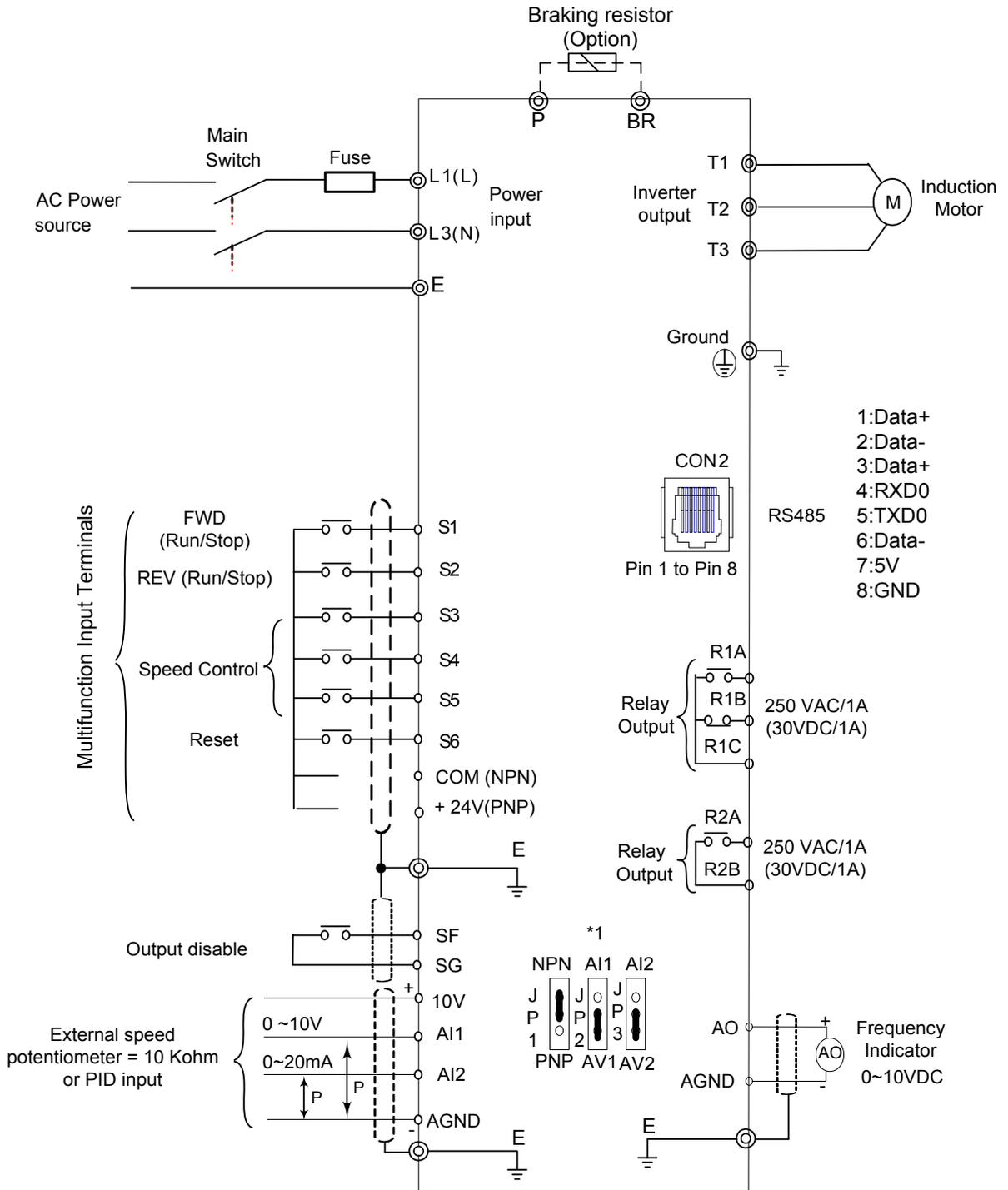
Ⓜ Indicates shield wire ⓂP Indicates twisted-pair shield wire
