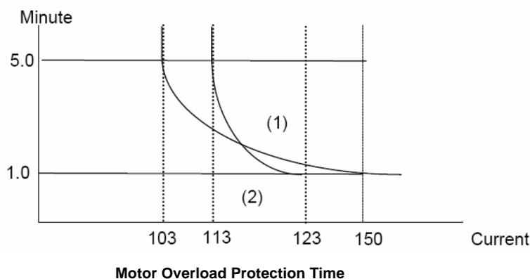
The heat sinking function will not be as effective when the motor run at low speed. So the thermal relay action level will decline at the same time. (The curve 1 will change to curve 2).
